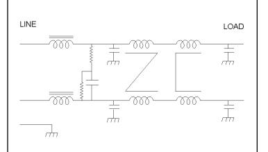
Diel. Withstanding (line - case) = \_\_\_\_\_1500 Vac Diel. Withstanding (line - line) = \_\_\_\_\_1500 Vdc
