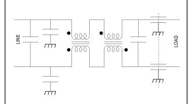
Operating voltage = 28—40 Vdc Operating current = 20 Amp
